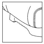
2. Place your hand under the front of the seat cushion and lift the cushion up while moving it forward. There is a label below the seat cushion with instructions to aid in seat operation.
